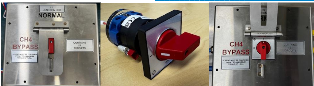
Figure 2. Example of CH 4 Switch and I.S. Junction Box
