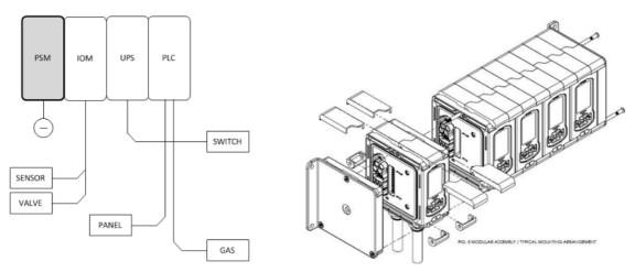
The assembly of the PSM module within a typically installed system is shown hereabove.
